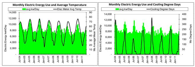
As can be seen above, close to 100% of thermal energy is dependent on weather for winter space heating. However, approximately 10% of electric use is dependent on weather and varies with summer temperature for air conditioning building cooling. The ratio of annual Wisconsin heating degree day comparisons to FY2005 base year provide an indication of anticipated weather adjustments for a building's thermal energy:
