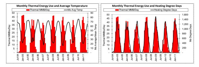
The relationships between electric energy use to degree days and temperatures for a sample facility (DOA-Milwaukee State Office Building) are shown graphically below:
