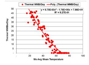
Similar methodology was used for weather adjustments presented in this report, but were based on second order polynomial equation curve fit. The same data above is plotted with at left with second order polynomial curve fit with a somewhat better R<sup>2</sup> than the linear equation in the above example.
