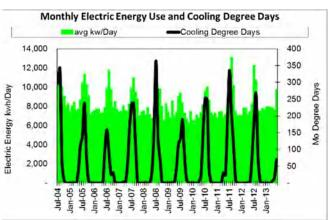
As can be seen above, close to 100% of thermal energy is dependent on weather for winter space heating. However, approximately 10% of electric use is dependent on weather and varies with summer temperature for air conditioning building cooling. The ratio of annual Wisconsin heating degree day comparisons to FY2005 base year provide an indication of anticipated weather adjustments for a building's thermal energy:
