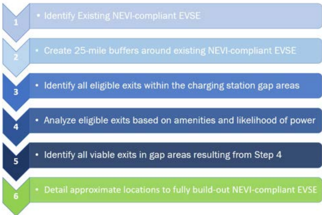
Figure 4-1: WEVI Plan Deployment Mapping and Process to Identify “Approximate Locations” of EVSE
