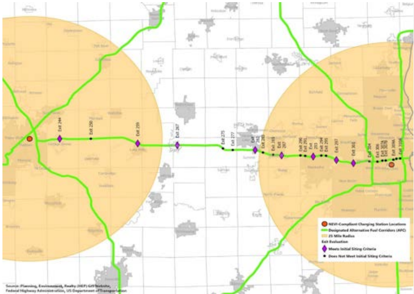
Figure 4-5: Example NEVI EV Charging Station Gap Area on I-94 between Madison and Milwaukee
