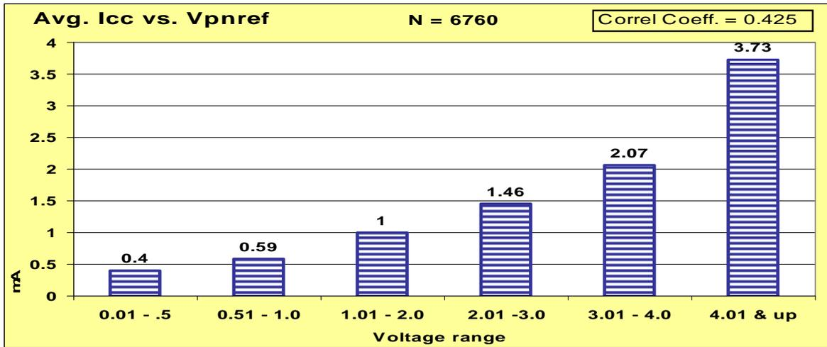
There is a significant statistical correlation between the average primary neutral-to-earth voltage and the average cow contact current. This is consistent with the electrical model that shows that  $V_p$  along with  $V_s$ ,  $V_{ps}$ , and  $V_d$  are the major contributors to animal contact currents.
