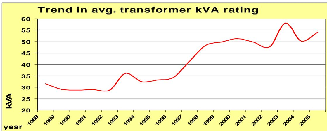
The trend clearly shows that the average size of dairy farms in Wisconsin is increasing, as the transformer kVA rating on the farms being investigated is increasing. From 1988 to 2005, the size of the average farm transformer's kVA rating increased 71%.
