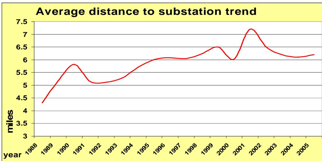
The trend indicates that in the early years of the SV program at the PSC, most farms that were investigated by the IOU's were closer to the substation. Recently, there is a trend to investigate farms that are farther away from the substation. From 1988 to 2005, the average distance has increased 44%.
