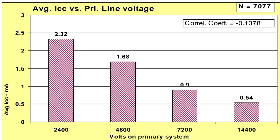
There is a distinct visual correlation to the relationship of primary system voltage level to average cow contact current. The mathematical correlation coefficient is moderate, but remember that the bar for 2,400 Volt only represents 0.5% of the systems and the next bar only 5.4 % of the systems reported.
