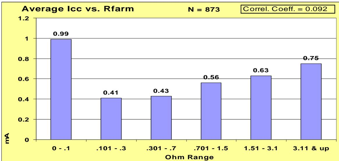
There is a very weak correlation coefficient between  $R_{\text{farm}}$  and average cow contact current. There are too few points reported at this time in the minimum range. One can assume that very resistive ground/neutral systems on farms have many alternate conductive paths for return currents but these paths may not always include the cow contact area.
