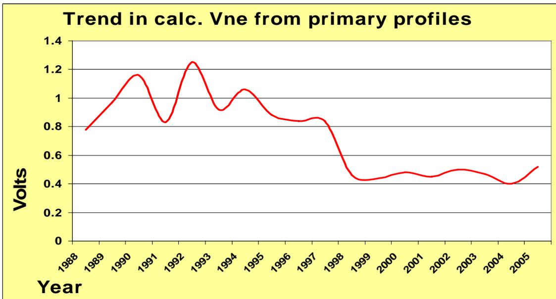
From 1988 to 2005, the calculated neutral to earth voltage on distribution pole ground rods has decreased 33%. To 2005, it has decreased 58% from the high recorded in 1992. The value has stayed within the range of 0.4 to 0.6 Volts for the last eight years.
