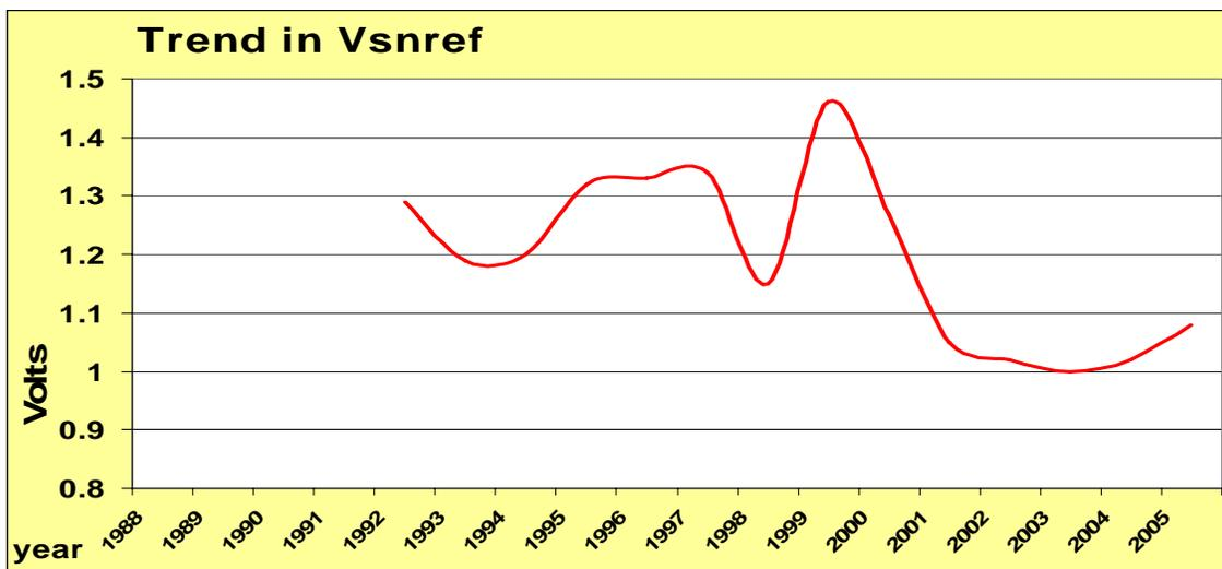
Overall, 95.1% of the readings are at or less than 3.0 Volts. The data was not recorded before 1992. From 1992 to 2005, the value of Vs has decreased an overall 16%. The trend was not favorable until after 2000 when the farm rewiring program was initiated. In the period from 1992 to 1999, it had actually increased 13%, but from 1999 to 2005 it has decreased 26%.
