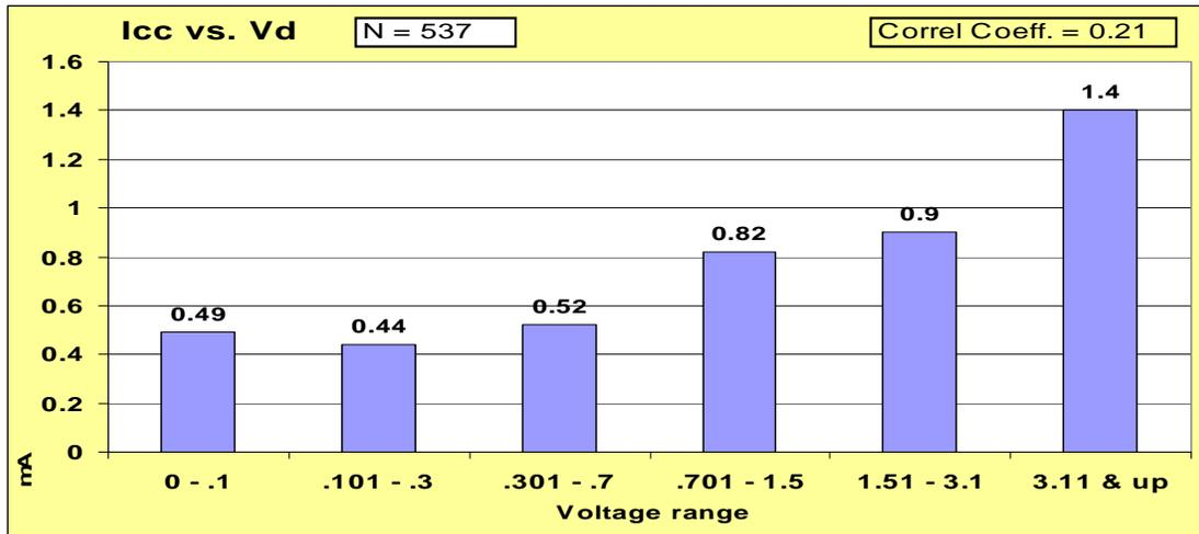
There is moderate correlation between the measured voltage drops and cow contact current, as one would expect. The data suggest that when the drop is 3.0 Volts or more, it can be a major contributor to elevated cow contact voltage.
