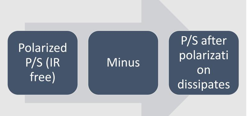
100 mV -Calculation Some pipelines depolarize quickly and others depolarize slowly.
