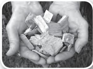
**Biomass** is organic matter (plant material, vegetation, agriculture waste, forestry waste) used as a fuel or source of energy. Use of biomass as an energy source results in little net production of carbon dioxide because the CO<sub>2</sub> generated during combustion of plant material equals the CO<sub>2</sub> consumed during the lifecycle of the plant. A map of biomass density across the United States can be found in the Map Appendix.
