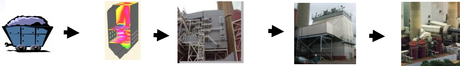
Fuel (low S) Burners (Low NO x ) Catalyst for NO x Precipitator (Particulate) Scrubber (SO 2 )
