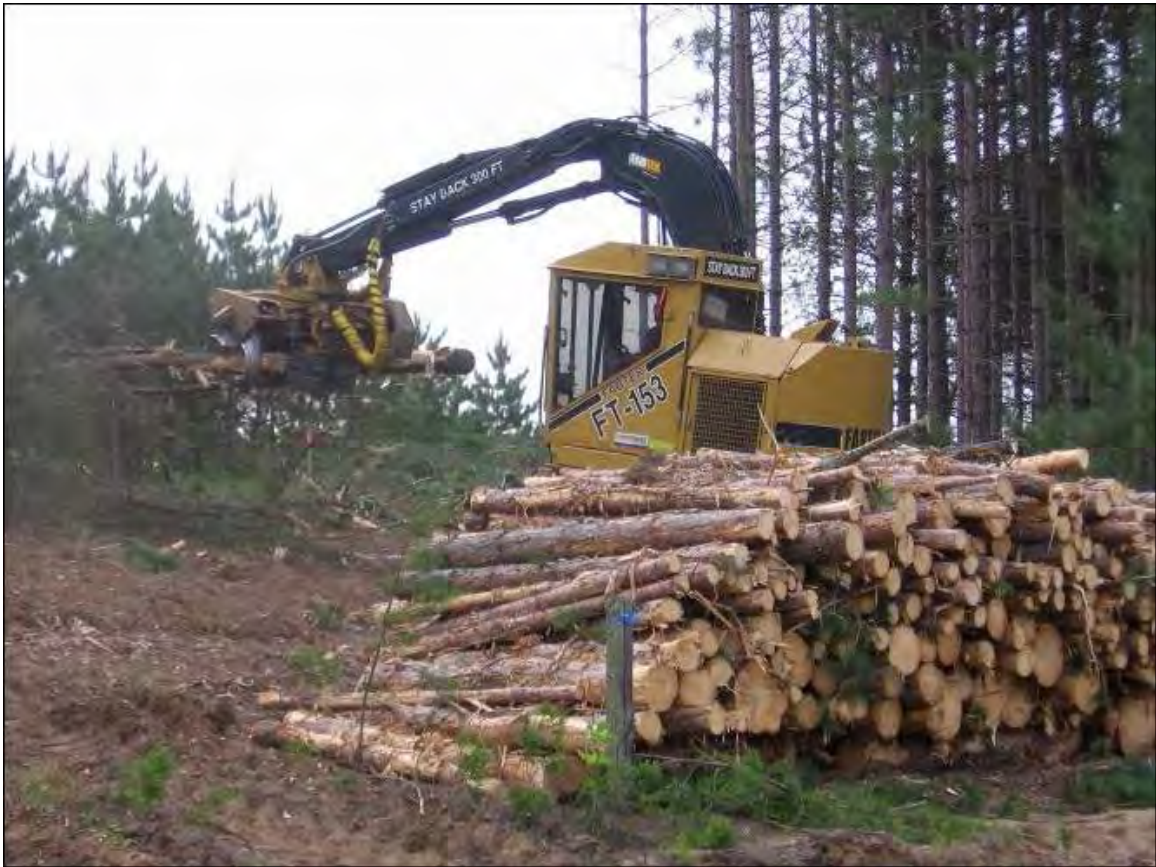
Figure Vol. 2-10 Tree processor used for clearing – capable of cutting a standing tree, de-limbing it, and sawing it into logs
